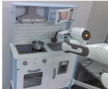
Figure 1: Visual example of the opening cabinet door skill in a real play kitchen environment. The agent has access to two visual representations, which we want to combine to a joint one for effective policy learning.
